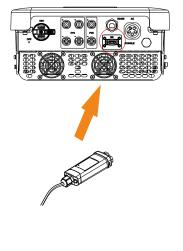
Plug the Pocket LAN into the correct port of inverter.
