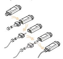
Remove the cover of DONGLE port at the bottom of the inverter. Ready to install your Pocket LAN.
